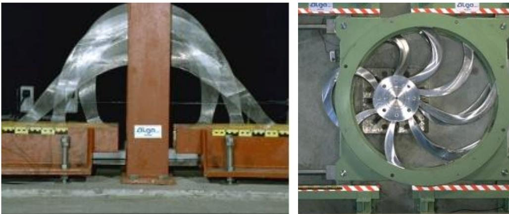
*Fig. 6-18: C-shaped Device (left) and EDU Device (right).*
