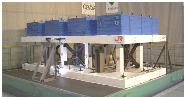
Fig. 11-71: Shake table test for the effectiveness of compression damper brace [Yoshida et al. (2005)]
