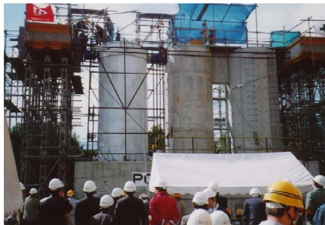
Fig. 11-36: On-site loading test on the effectiveness of PC segment jacketing
