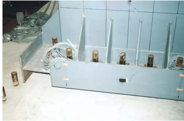
Fig. 11-9: Test models (9m tall and 2.5m x 2.5m section) for steel jacketing with controlled enhancement of flexural capacity
